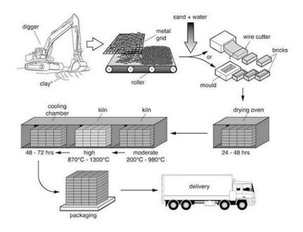
The flow chart shows the way in which bricks are made for the building industry.
